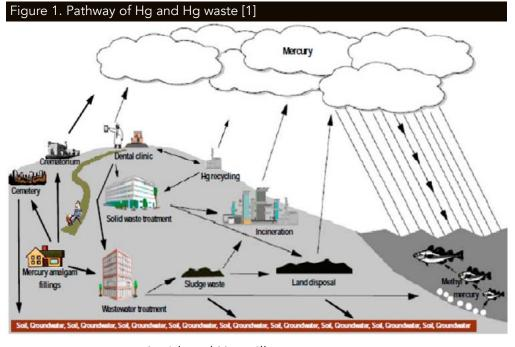
Figure 1 illustrates the general flow of Hg through the dental clinic or laboratory and downstream. While it shows how Hg wastes join the general waste stream and enters the environment, it does not include Ha emissions to the air which may occur in various stages during handling and placing of Hg amalgams or as releases from the wastewater system. Dental personnel may be exposed to the different sources of Hg vapors in the duration of [19]:
